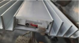
**6)**Install the extrusion on the coach ceiling.
